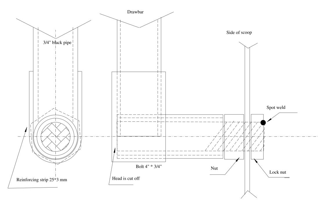
Drawbar attachment to Scoop Body D 3A
